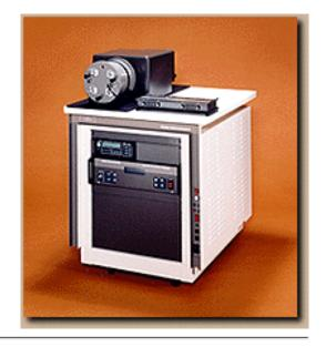
The Pulse Instruments MODEL PI-4880 FLOOD BEAM OPTICAL TEST HEAD is a transportable, turnkey subsystem that provides a controlled optical flux and temperature environment test head for the testing of IR Detectors and Focal Plane Arrays. Modular design and a host of options allow a maximum of configuration flexibility at a minimum cost. Ergonomic design and user friendly software maximizes test throughput and minimizes set-up time.
