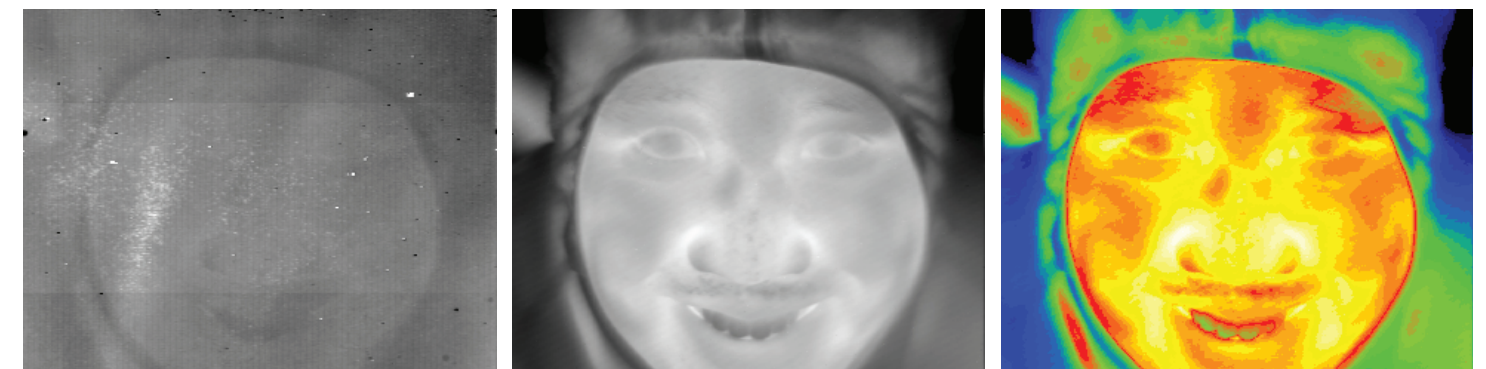
Fig. 2: Uncorrected and Fully-Corrected Images Acquired by PI-3105
